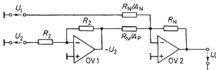
Drawing 2 - Subtraction circuit using the adder circuit
