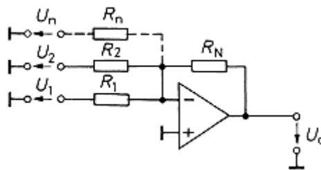
Drawing 1 - Inverting adder circuit
